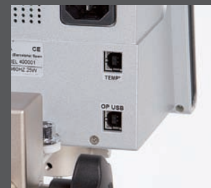
Rear view to the viscometer showing the new USB interface that provides a faster transfer of data to the computer.
